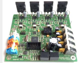
**5004B-EP350 - DMX Current Source 24VDC 4x350mA
