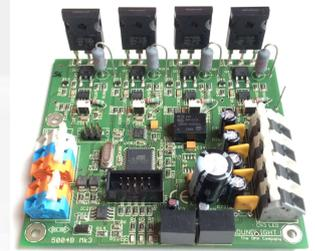
**5008A-EP - LED Driver 8-Channel 24V PWM0,5A
